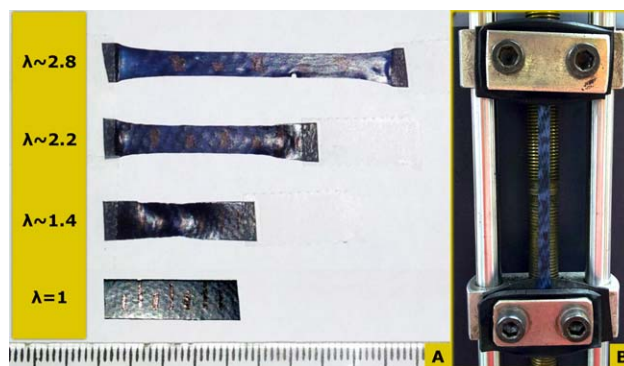
Figure 3. Images of (A) Maxon SC-MP_C samples (thermally treated for 1 day at 75 °C) drawn at various draw ratios and (B) a sample of the same batch drawn at \lambda \sim 4 held at the grabs of the stretching device. [Color figure can be viewed in the online issue, which is available at wileyonlinelibrary.com .]
